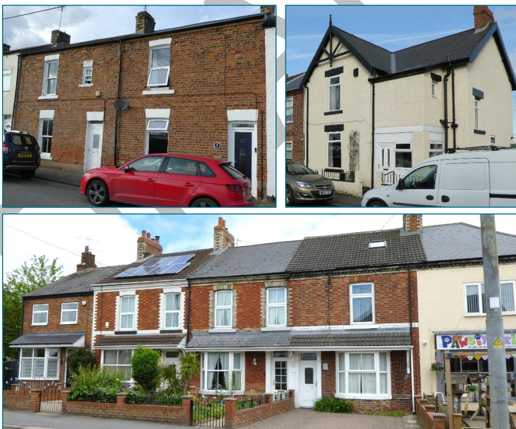
Subzone D2: Top left: A few of the well-preserved houses of Killinghall Row, which face directly onto the pavement. Top right: Gable-fronted end unit of terrace along Middleton Lane. (Photos © Gaby Rose, March 2024) Bottom: Terrace at southern end of Station Road with polychromatic brickwork. The once continuous roof surface has now been broken up by using different materials. (Photo © Gaby Rose, May 2024)
